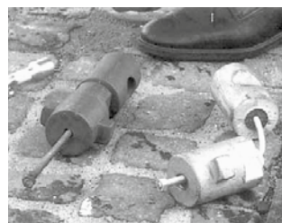
4 | Junction piece: damaged (right) and replacement (left)
