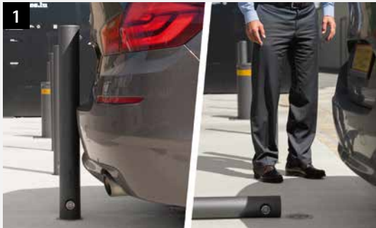
Bollard hit by a car. The replaceable junction piece breaks at the predetermined breaking point. The bollard and foundation with base generally remain intact.
