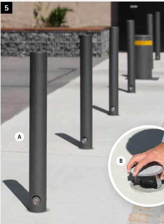
A) Bollard back standing firmly once more B) When the bollard is removed, the ground shell can be closed with a cover
