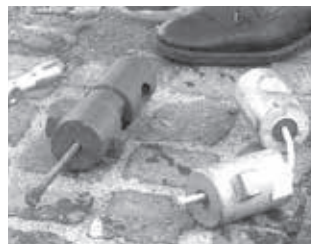
4 | Junction piece: damaged (right) and replacement (left)
