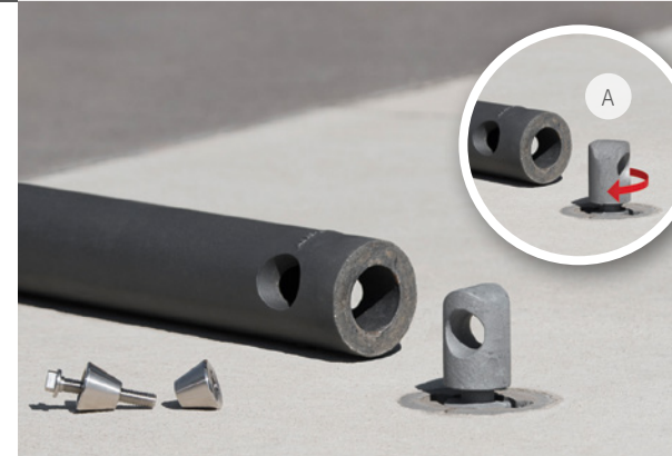
A Insert a new junction piece in the ground shell and turn it by 90°
