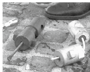
4 | Junction piece: damaged (right) and replacement (left)
